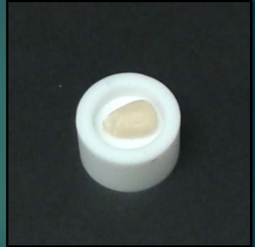
Hollowed out Teflon disk with maize kernel
